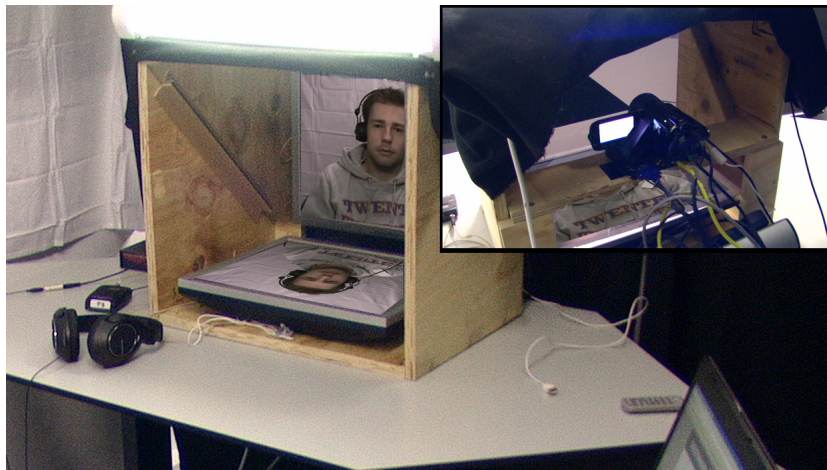
Figure 2.1: Picture of the cubicle in which each participant was seated. It illustrates the interrogation mirror and the placement of the camera behind it which ensures eye contact.
